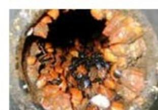
▲ Eroded water pipe due to the propagation of marine organisms
